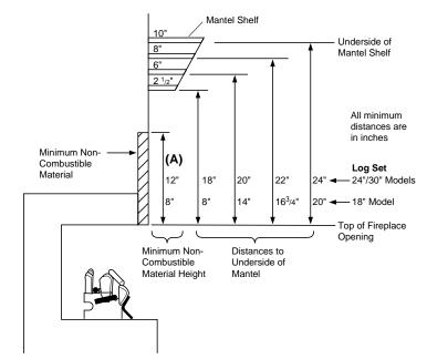
Figure 7 - Minimum Mantel Clearances Without Using Hood
